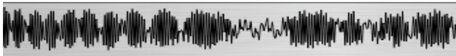
Figure 2: Difference between the two angles q_1 and q_2 at a range of calculation steps in the simulation run for the Poincare plot. See the next section for details.
