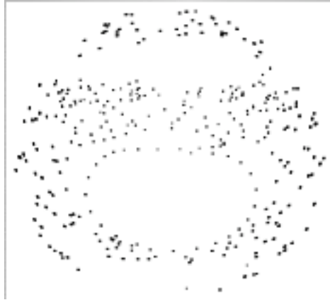
Figure 3: Poincaré plot of the simulation run "DP10" (see appendix for details). On the abscissa, the angle q_1 is drawn, and on the ordinate the momentum p_1 . For the plot, the program was slightly modified, in order to spare calculation time: artificial jumps were built in, whenever the angles exceeded 2\pi . Then, p_2 was set to zero and p_1 accordingly calculated out of the energy function ( p_1 = f(q_1, q_2, h_0) ). This helped starting again at different states of the phase plot, and provide a more complete picture.
